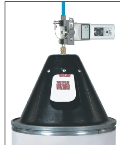
HHSS at the drum side of the conduit run
